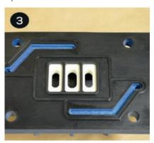
Insert the (4) cap screws & washers (items 1 & 2) through the valve body and
