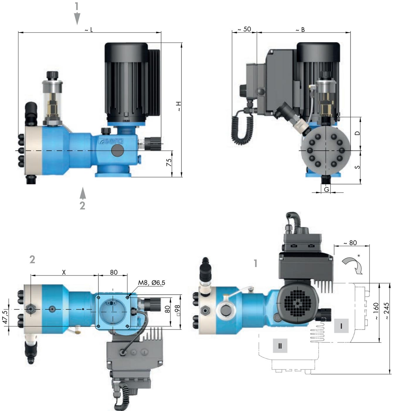
\* Drive with electronics can be rotated throughout  $90^\circ$  each and can be put to the positions I and II. (release the motor fastening screws, put the motor carefully to the desired position and fasten with screws again).
