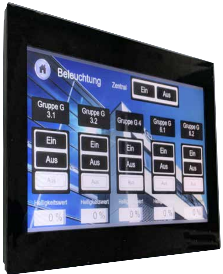
KNX display for setting the various different light areas
