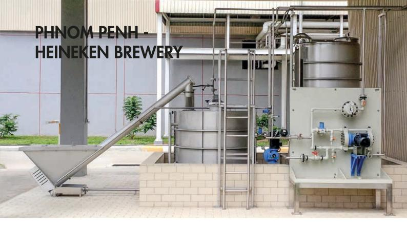
Approximately 50 million tons of caustic soda are produced annually and used in various ways in industry. **sera** has developed a cost-effective system solution specifically for use in the food industry, which has a variable but large demand for alkaline cleaning agents such as caustic soda. This enables safe and efficient preparation of caustic soda based on sodium hydroxide (NaOH) in solid form (pellets, flakes, pearls or powder) and water.
