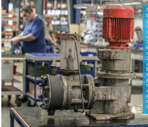
family The Dinkelacker brewery, founded in Stuttgart in 1888, has been using sera dosing pumps for a hygienically perfect brew-ing process for decades. The R413KM was used to dose chemicals in the cleaning process for over 30 years – but the wear and its age could no longer be ignored and a replacement was essential. As this pump was removed from our product range several years ago, our Service department recommended reconditioning the old pump as a solution.
