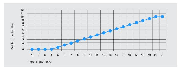
The stroke speed is set in the same way as for the batch quantity. First select the maximum value that corresponds to the 20 mA signal. The delivery rate can now be set using an appropriate input signal between 4 mA and 20 mA.
