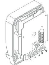
■ Insert the mains pipe through the cable fitting M20 from below into the housing.
