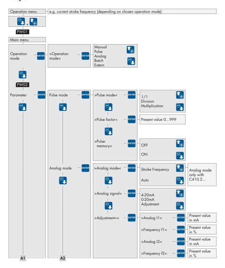
PW01 Locking by Password 01 (pre setting ex work: 9990, not activated)
