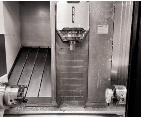
Spindle unit for axial and radial machining
