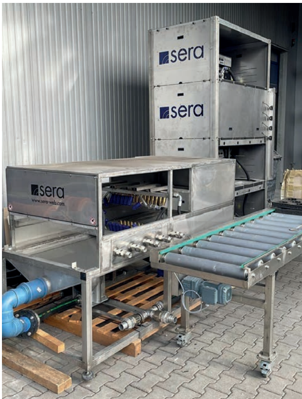
Customised continuous system for cleaning special profiles for powder coating.
