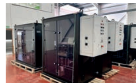
sera supplied 14 dosing systems with a total of 40 diaphragm dosing pumps, equipped with control cabinets and Profibus DP communication.
