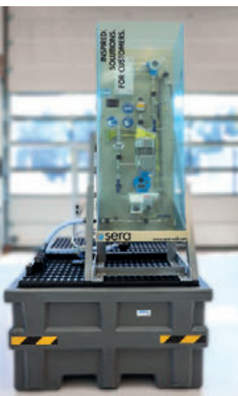
Dosing station for caustic soda: Removal of the medium from the on-site IBC and dosing into the high-pressure area.
