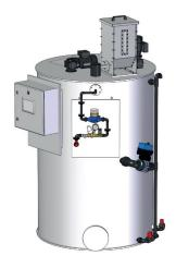
Fully automatic preparation of organic flocculent aid (pulverized and/or liquid) Process logic control (PLC) Selectable concentration of prepared solution Feeding device Dry material feeder with thermal protection zone Pump for liquid polymer (option) Dissolving water unit
