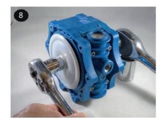
Install the liquid chambers (item 18) by placing one side over the diaphragm. Start all 6 screws (item 11) before tightening and torqueing. Torque all fasteners in a star pattern to 50 in-lbs (5,6 Nm). Start all 5 screws (item 17) before tightening and Torqueing. Torque all screws in a X Pattern to 30 in-lbs (3,4 Nm). Repeat to install the second liquid chamber. Ensure both chambers are orientated the same and that the inlet and outlet ports are vertical when facing the front of the pump.
