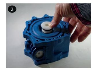
If replacing the bushings (item 24), then the muffler felt (NS) should also be replaced prior to replacing the second bushing. It is important when installing the felt that it does not block the air slot. Lubricate the bushing orings (item 25) and press it into the open bushing gland. Reinstall the bushing, hold down screw (item 17).
