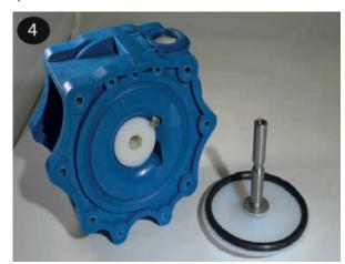
For PTFE fitted pumps place the large diaphragm o-ring (item 21) into the groove in the center section (item 28).
