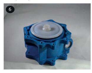
Tighten and torque the outer plates (item 19) to 40 in-lbs (4,5 Nm).
