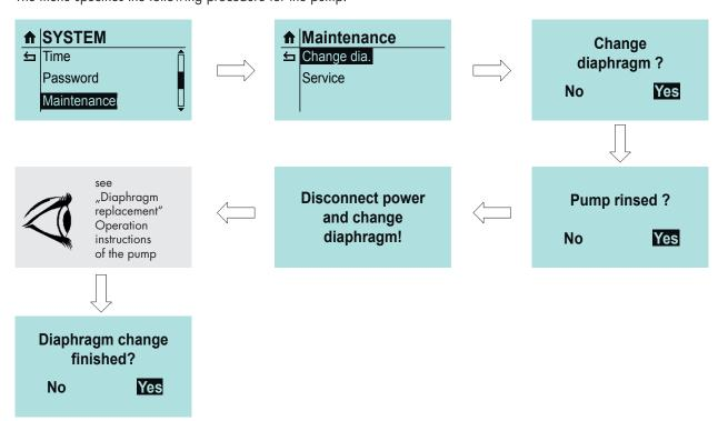
The counters for diaphragm operating hours and diaphragm service life are reset after successful diaphragm replacement.
