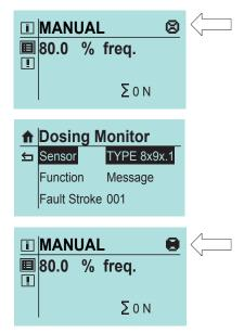
If no flow is detected, the error message "No flow present" is displayed after executing the specified number of fault strokes. The ring initiator must then be pushed upwards slowly.
