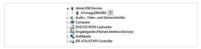
Store the folder with the "USB-Update vM01.00X" update files on the drive where the installation of Atmel FLIP was saved. Start the "USB\_run\_vM01.00X.bat" batch file in the folder by double-clicking it.
