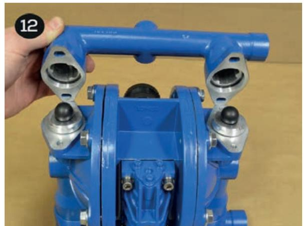
**AIR END SERVICING (INSTALLING AIR END KIT)**
