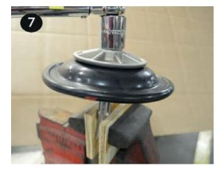
After performing required maintenance, the pump can be reassembled. The pump can also be reassembled using the disas-sembly instructions in the reverse order as listed above. For detailed assembly instructions, follow the steps in the Wet End Reassembly section "MONTING" beginning on page 16.
