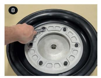
After performing required maintenance, the pump can be reassembled. The pump can also be reassembled using the disassembly instructions in the reverse order as listed above. For detailed assembly instructions, follow steps in Wet End Reassembly section "MOUNTING" beginning on page 16.
