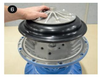
It may be easier to thread the outer plate (item 20) onto the shaft (item 33) if the diaphragm(s) is inverted on one or both sides. This can be done by hand.
