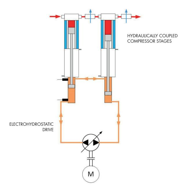
The compressor unit consists of two coaxially arranged vertical gas cylinders, each mechanically connected to and driven by a hydraulic cylinder.
