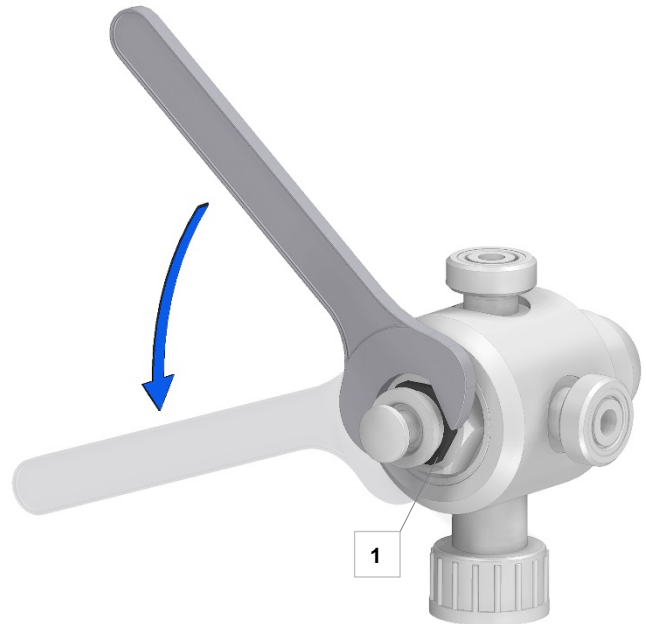
Fig. 13 Pressure adjusting of relief valve
