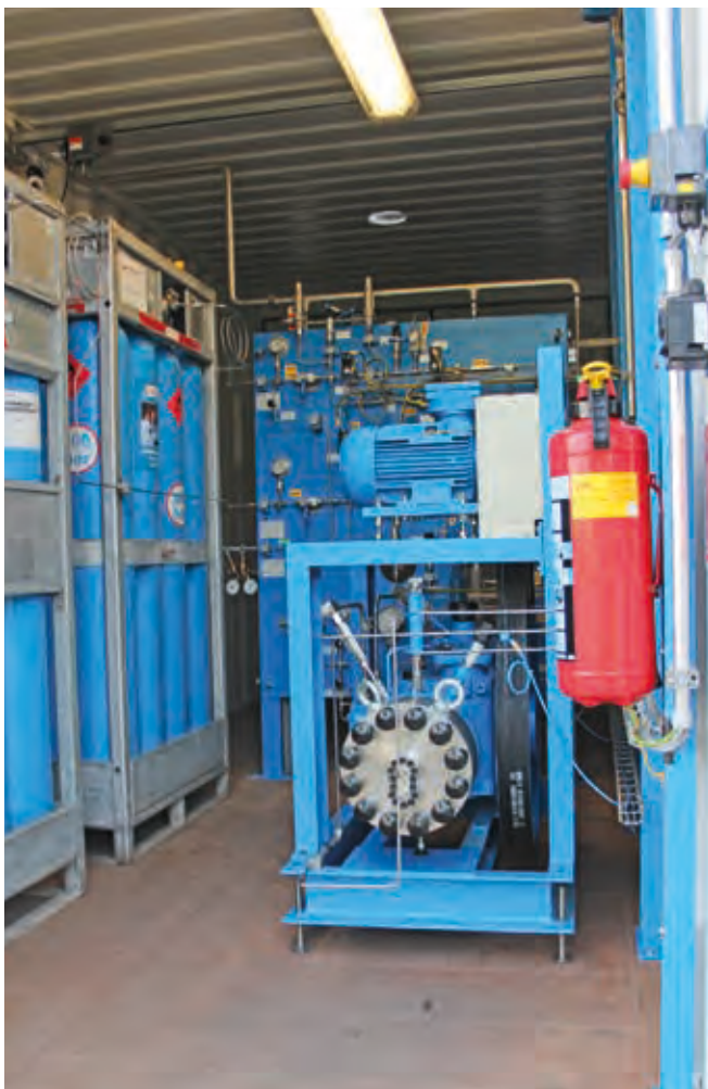
Standard compact diaphragm compressor with cylinder bundles
